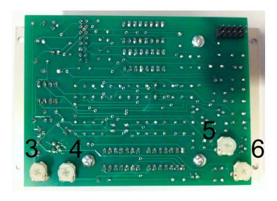
Trim pots 3 and 5 have direct control over the quality of the delay signal. The delay will work within a small range of the trim pots. The best sound quality is available when the trim pots are set to the middle of this range.
