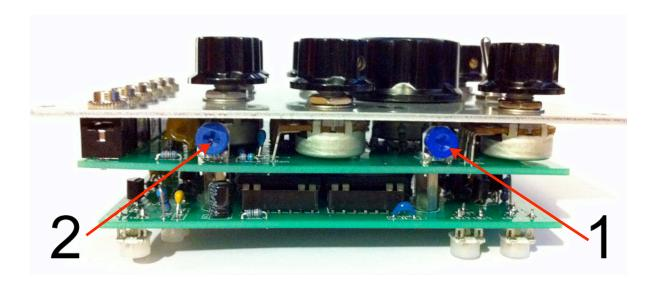
The trim pot closer to the top of the module (1) is the main control for setting the maximum delay length. The second trim pot (2) adjusts the range of the delay length available from the rate control and also affects the delay length.
